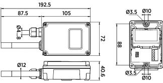
HMD82/83(D) RH+T and TMD82 T-only transmitters for ducts
