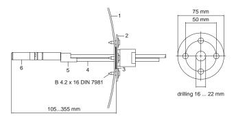
Duct installation kit **10697** (215003 for HMT337 temperature probe)
