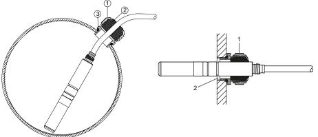
$\label{eq:hmp247CG: Vapor-tight installation with cable gland} \textbf{HMP247CG: Vapor-tight installation with cable}$
