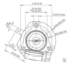
Probe mounting flange, side and front view
