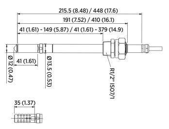
Optional filter for low pressures, suitable for all models, dimensions in mm (inches). Optional filter provides faster gas exchange to the sensor in applications where protection from particulates is not needed.
