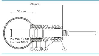
Pressure-tight Swagelok installation kits **SWG12ISO38** with ISO3/8" or **SWG12NPT12** with NPT1/2" thread (SWG6ISO18 with ISO1/8" or SWG6NPT18 with NPT1/8" thread for HMT337 temperature probe)
