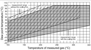
Dew point accuracy vs. measurement conditions
