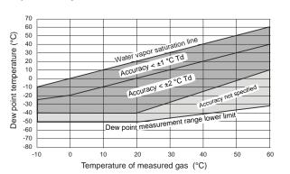
Accuracy (A probe)  $-40 \dots +60 \, ^{\circ}\text{C}$   $\qquad \pm 2 \, ^{\circ}\text{C} \, (\pm 3.6 \, ^{\circ}\text{F})$  (see graph)
