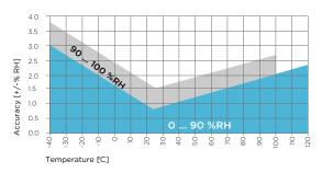
HMP9 humidity measurement accuracy as a function of temperature
