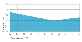
HMP1 temperature measurement accuracy over full range
