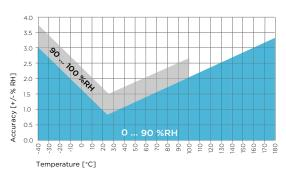
Humidity measurement accuracy as function of temperature
