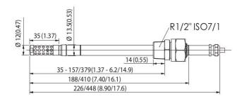
MMT318 probe, dimensions in mm (inches)
