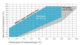
Dew point accuracy vs. measurement conditions
