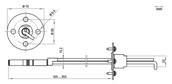
Duct installation kit 210697 dimensions with probe
