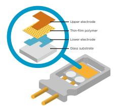
Structure of the HUMICAP sensor
