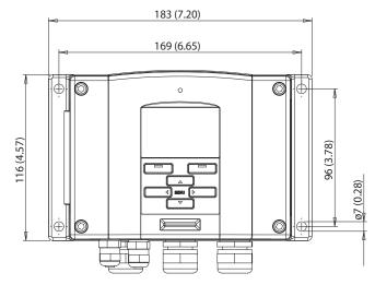
DMT345 and DMT346 Transmitter Housing
