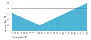
HMP4 temperature measurement accuracy over full range
