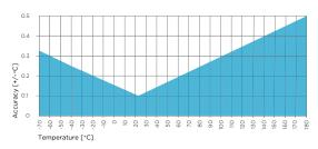
HMP8 temperature measurement accuracy over full range
