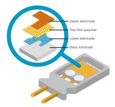
Structure of the HUMICAP sensor
