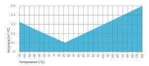
HMP7 temperature measurement accuracy over full range
