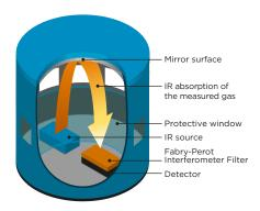
Structure of the CARBOCAP sensor
