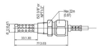
MMT317 probe, dimensions in mm (inches)
