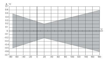
Temperature measurement accuracy over temperature range
