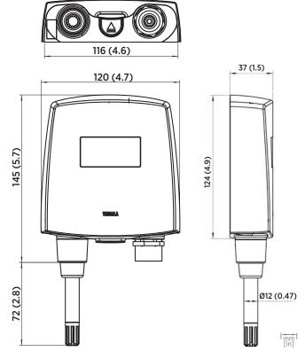
Dimensions of remote probe (top image) and HMT120, HMT130, TMT120, and TMT130 transmitters
