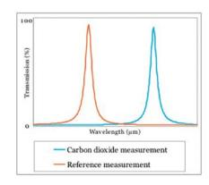
Example of carbon dioxide measurement. Both reference and CO2 absorption are measured in the same optical path
