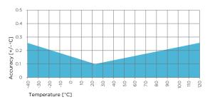
HMP9 temperature measurement accuracy over full range
