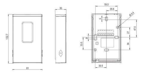
Dimensions (in mm) of GMW90 series transmitter cover (left) and mounting base (right)  $\frac{1}{2}$
