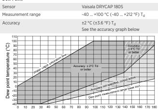
Dew point accuracy vs. measurement conditions
