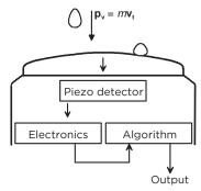
Pv = vertical momentum m = mass of drop v, = terminal velocity of drop
