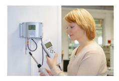
Handheld Humidity and Temperature Meter HM70 is ideal for field checking HMT330 transmitters
