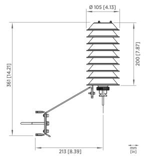
Solar Radiation Shield DTR502B dimensions
