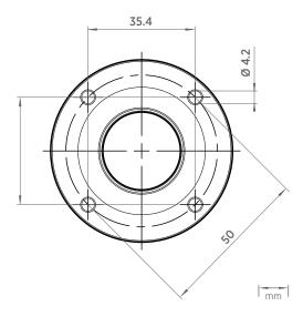
Dimensions of probe mounting flange (243261SP)
