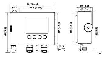
HMT370EX dimensions in millimeters and [inches]
