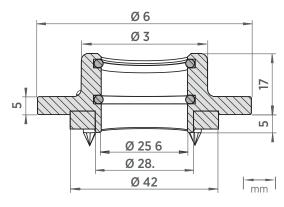
Probe mounting flange dimensions, cross section
