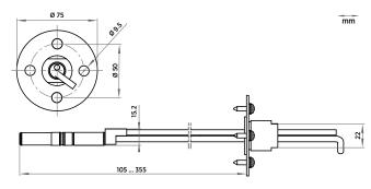
Duct installation kit 210697 dimensions with probe
