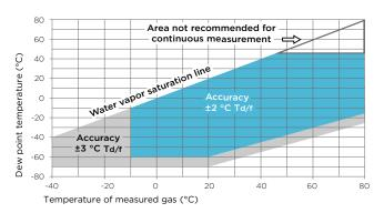
Dew point accuracy vs. measurement conditions
