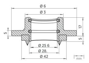
Probe mounting flange cross section
