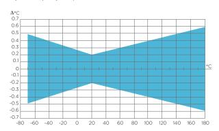
Temperature measurement accuracy over temperature range
