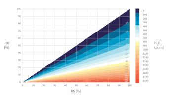
For example, at 20 °C and 500 ppm hydrogen peroxide, the humidity level 25 %RH is equivalent to 60 %RS. When this gas mixture starts to condense (relative saturation being 100 %), relative humidity is 45 %.
